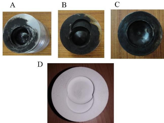
**Figure 1: Pictorial view of Standard Toroidal Geometry (A), Shallow toroidal Re-entrant Geometry (B), Hemispherical Open Geometry (C) and Shallow toroidal Re-entrant Geometry-LHR piston**
