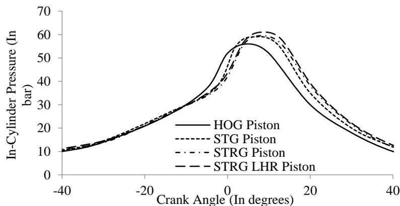
**Figure 3: Variation in In-Cylinder pressure for HOG, STG, STRG and STRG LHR piston at full load**
