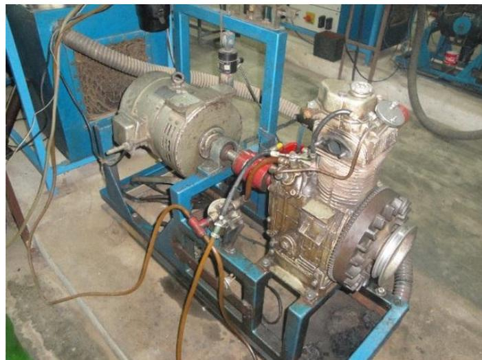
**Figure 2: Pictorial view of Test Engine**
