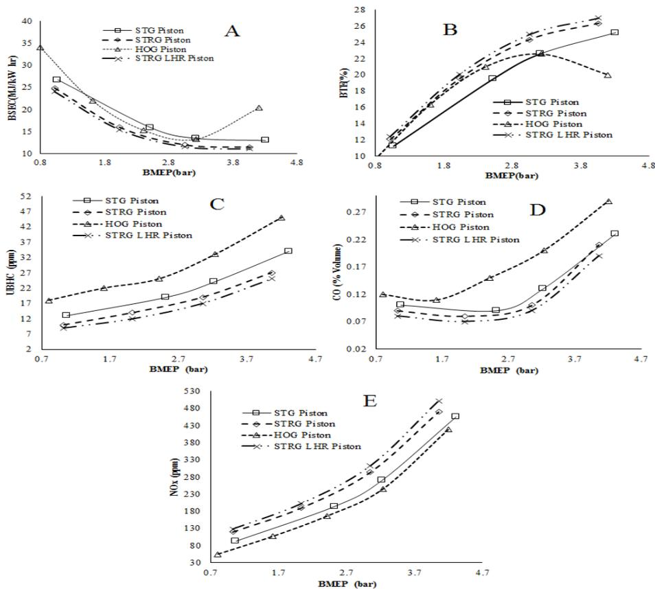
Figure 5: Variations of BSEC (A), BTE (B), UBHC (C), CO(D) and NO<sub>x</sub>(E) with BMEP for STG, STRG, HOG and STRG LHR pistons
