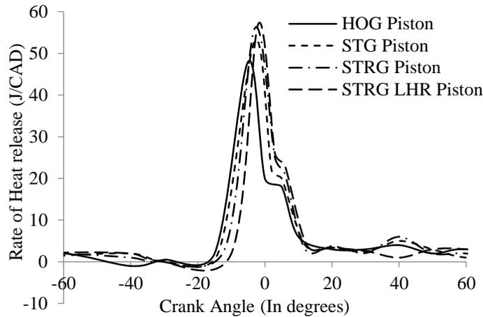
Figure 4: Variation in Heat release rate for HOG, STG, STRG and STRG LHR piston at full load
